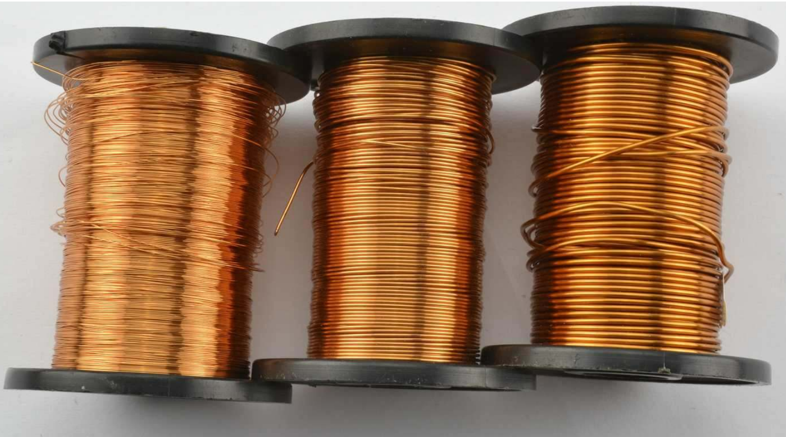
Figure 2-12. Enamel-Insulated Wire for Winding Inductors 30-22 AWG
