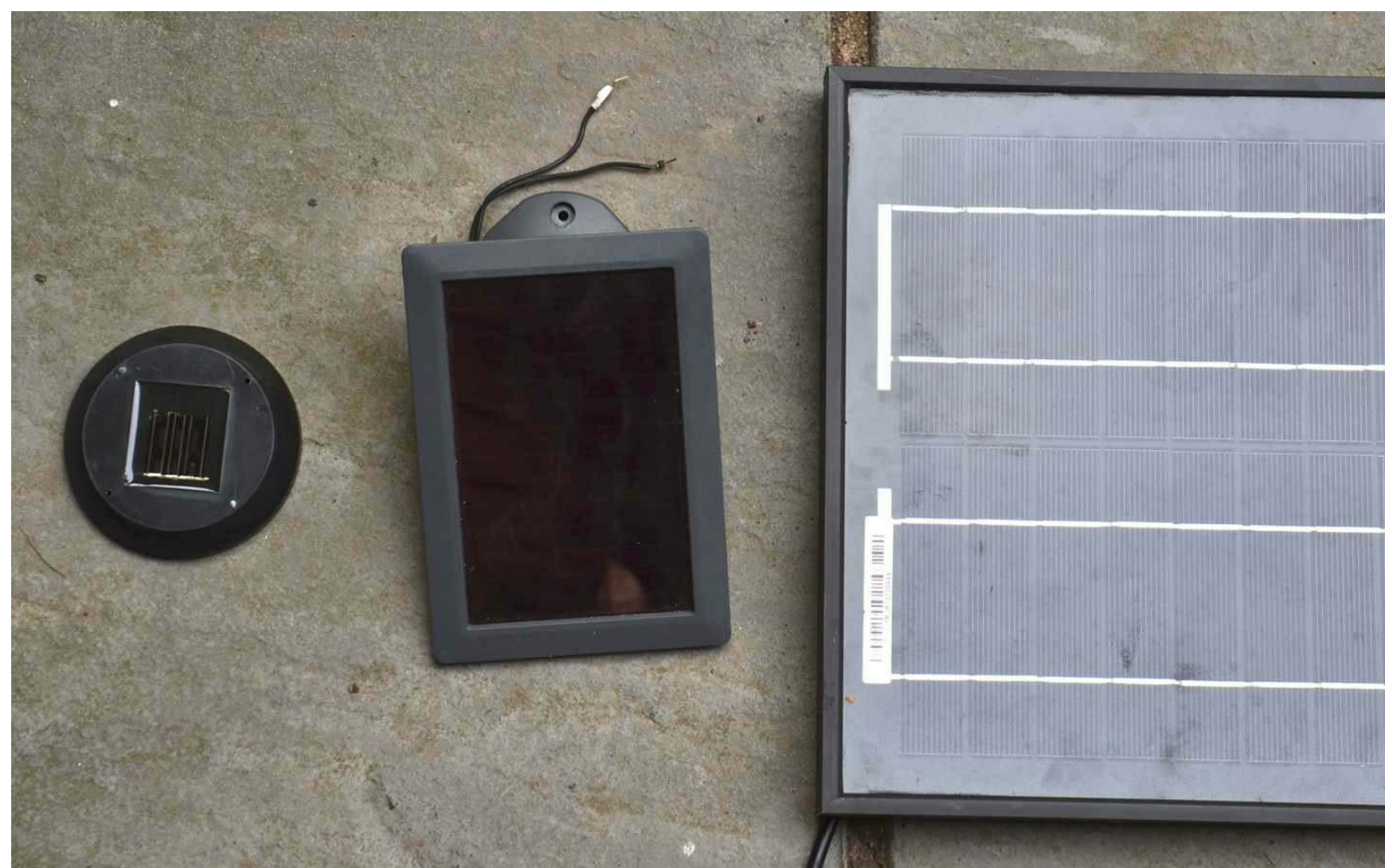
Figure 9-1. A Selection of Solar Panels — Left to Right Unknown Wattage, 1W, and 20W Panels
